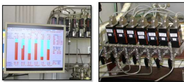
Figure 2: Custom-made interface used to control the gases flow rates (left panel) through Mass Flow controller (MFCs, right panel).
